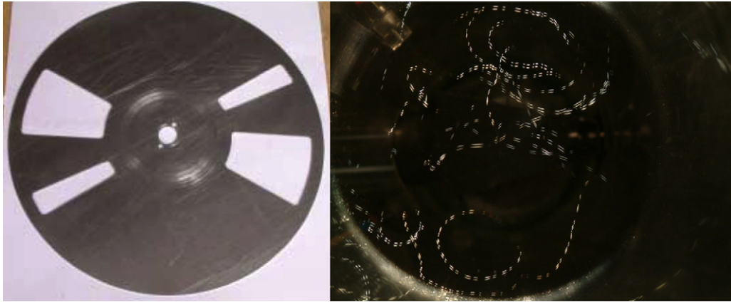
Fig. 13. Left: the screen rotated in front of the continuous white-light source to generate coded streaks from the tracer on photographic images. The light was caused to form a sheet by a second, stationary, screen. Right: an example of the resulting images.
