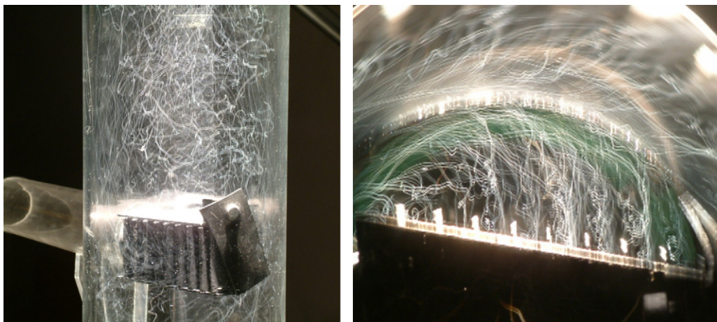
Fig. 8. Flow around the vaned inlet to a gas scrubber. The internal diameter of the cylinder housing the inlet is 150 mm. To the right, the whole vaned inlet assembly is seen, with the flow from the vanes at the side, continuing in a rather turbulent by evenly distributed manner above the vane. To the left a detail of the flow emanating from the vanes.
